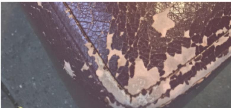
The photograph above shows a hydrolysis related failure of a low grade Polyurethane in a restaurant installation after 18 months of use.
